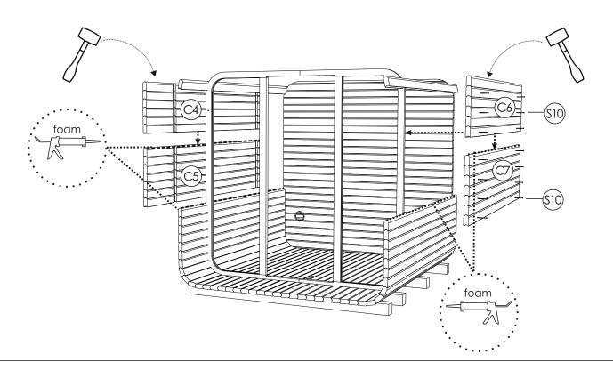
**STEP 10:** Fix the next body staves (C; C1) and board panels (C2;C3) on both sides with foam between the stave and panel with screws 4x60(S10) for each side. Use a rubber hammer if necessary, possibly need to push a bit back and front panels.
