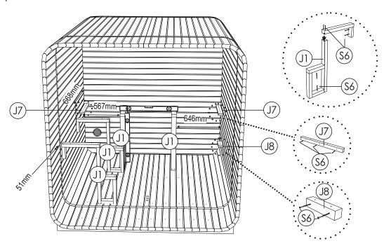
**STEP13:** Install sauna benches on top of legs (J; J3; J4; J5). Bench cross boards have to match the tops of the bench legs. Check distances from walls, then fix benches on the legs.
