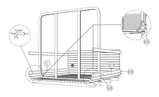
**STEP 7:** Fix the next board panels (C4; C6) on both sides with foam between the stave and panel with screws 4x60(S10) for each side. Use a rubber hammer if necessary, possibly need to push a bit back and front panels.
