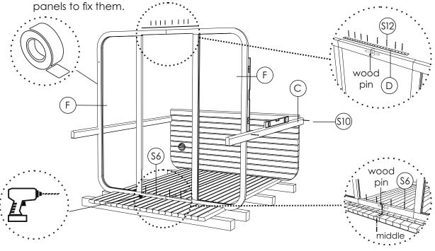
**STEP 6:** For both sides, the 10th to 11th stave (C) needs to be fixed as one piece. One is holding those three staves, and the other is fixing only the 12th; 13th; 14th; stave with screws 4x60(\$10). Between floor panel and every stave use foam for better insulation.
