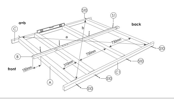
**STEP 2:** Drill 10mm hole in each plank,in the front wall groove and in the rear wall groove to the out-side. Fix 2 board panels (C2; C3) with 5x100 ss screws (S1) to each side from the centre stave. Use 8 screws for each panel as shown in picture. Between panel and stave use foam for better insulation.
