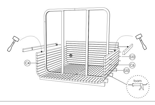
**STEP 8:** Install the upper rear panelsl (V3;V4) with caution. Use foam between panels for insulation. Place it on top of the back panel. Check that side edges are aligned properly with both panels. One keeps holding the panel in line, and the other is fixing the staves (C; C1) on each sides curve using screws 4x60(\$10). Check levels and fix the panel with screws at the ends of the panel's lower sides using screws 5x120(\$4).
