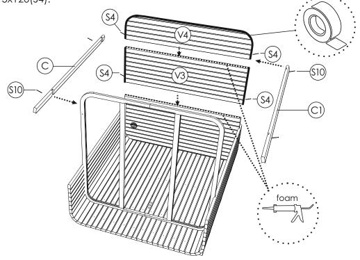
**STEP 9:** Fix the next board panels (C4; C5; C6; C7) on both sides with foam between the stave and panel with screws 4x60(\$10) for each side. Use a rubber hammer if necessary, possibly need to push a bit back and front panels.
